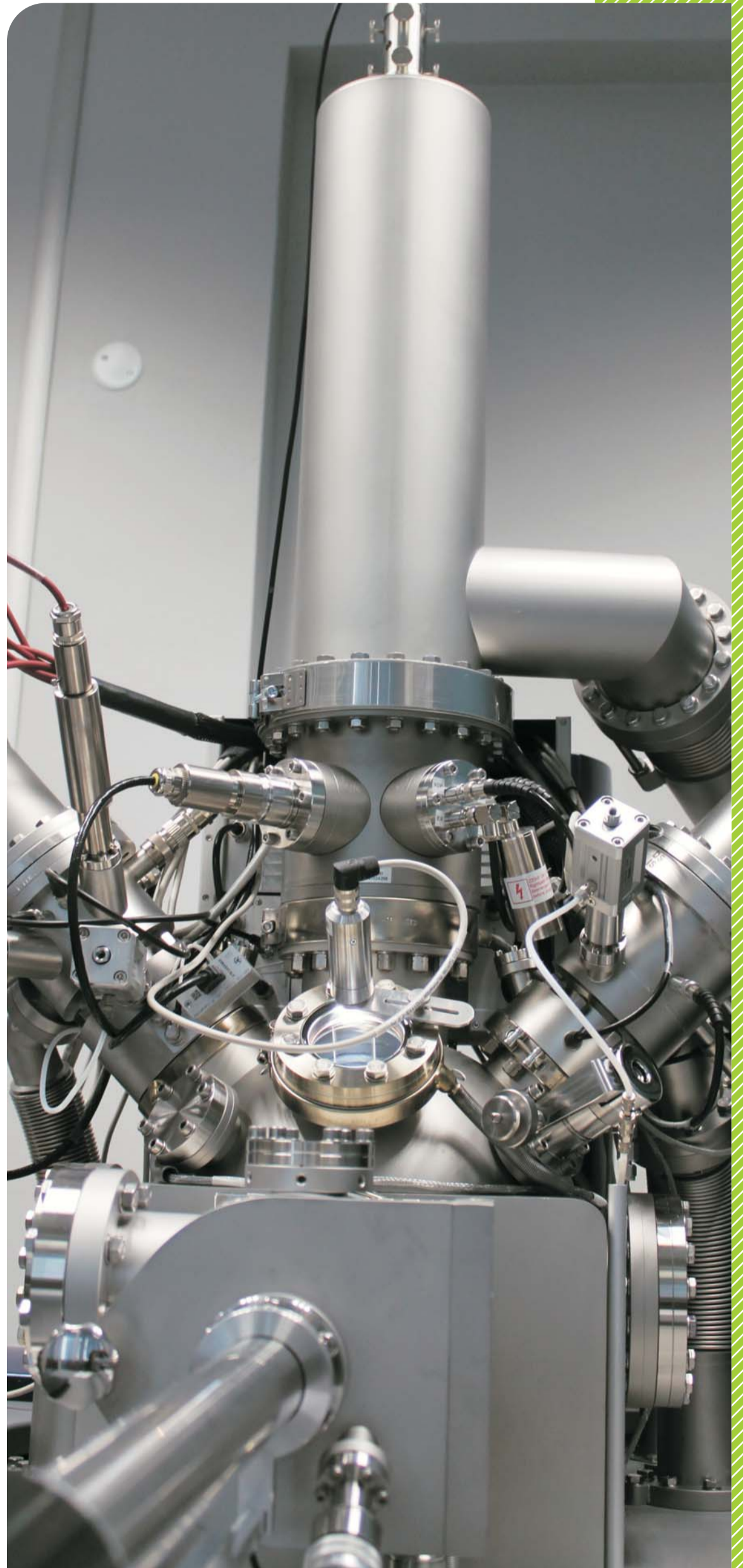
The Time-Of-Flight-Secondary-Ion-Mass-Spectrometer (TOF-SIMS)
