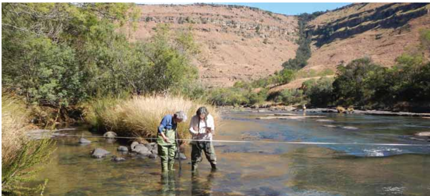
Measurement of streamflow by Laura Bannatyne and Kate Rowntree in the Tsitsa river, Eastern Cape, which forms an important tributary of the Mzimbvu River, a project examining catchment processes that will support catchment restoration aimed to reduce sediment yield in river systems. Photo: B. van der Waal
