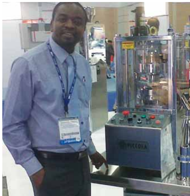
Dr Sandile Khamanga, senior lecturer in the Faculty of Pharmacy, is seen here with a Table Press, which is used in the manufacture of tablets.
