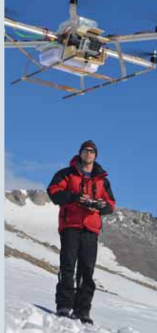
David Scott (Masters Student) in the Jutulsessen area of Antarctica flying a UAV (Unmanned Airborne Vehicle) which he built with Dave Forsythe (Institute for Water Research) to photograph and map the landscape in three dimensions
