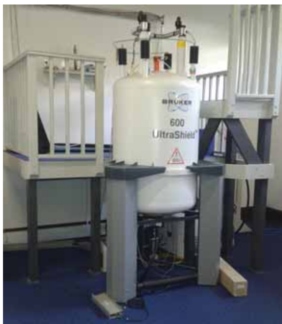
Cryoprobe 600 MHz NMR, used for: 1D and 2D analysis of solutions Photo: Jethro Christian
