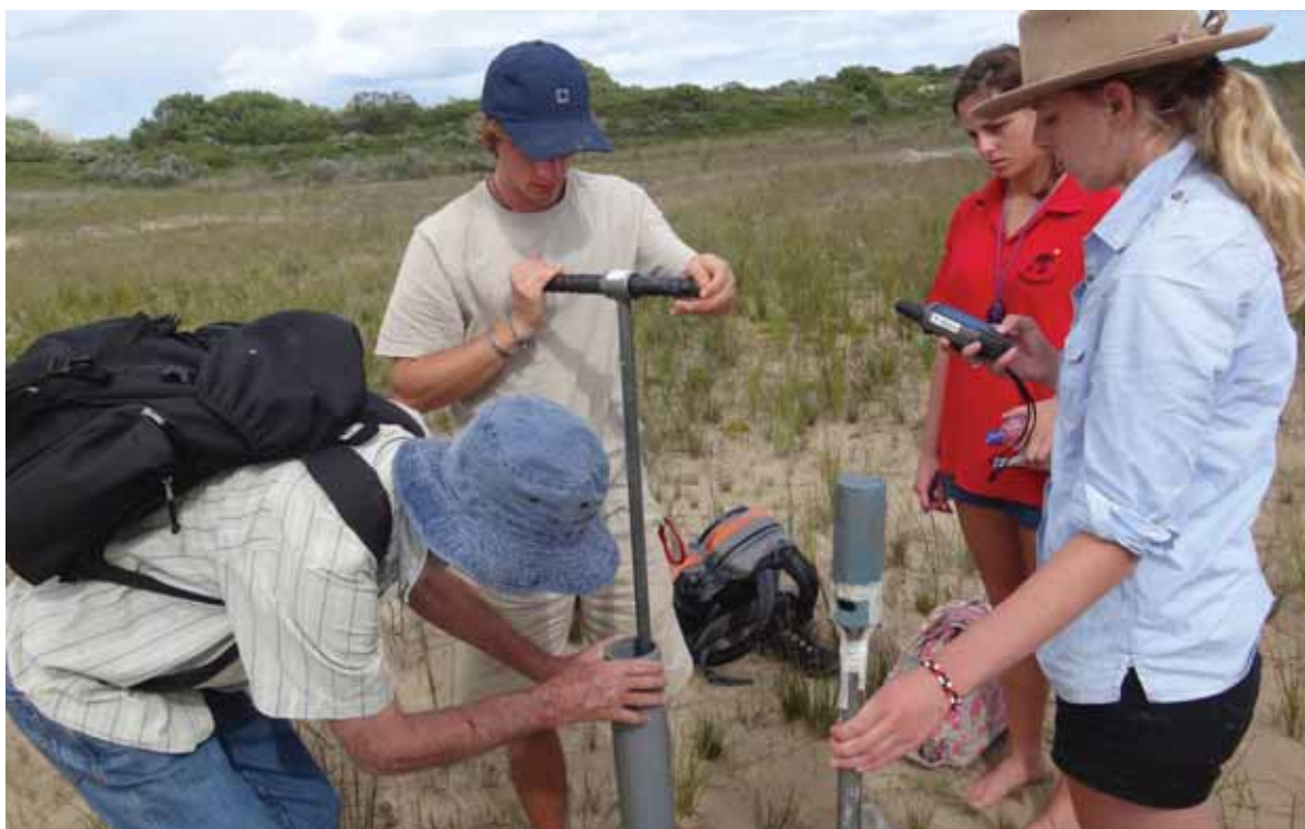
From the left: Professor Fred Ellery with Honours students, Nicholas Huchzermeyer, Amy Barclay and Philippa Schlegel, installing a piezometer in the Sand River wetland near St Francis Bay, to measure daily water loss due to transpiration by alien plants further upstream
