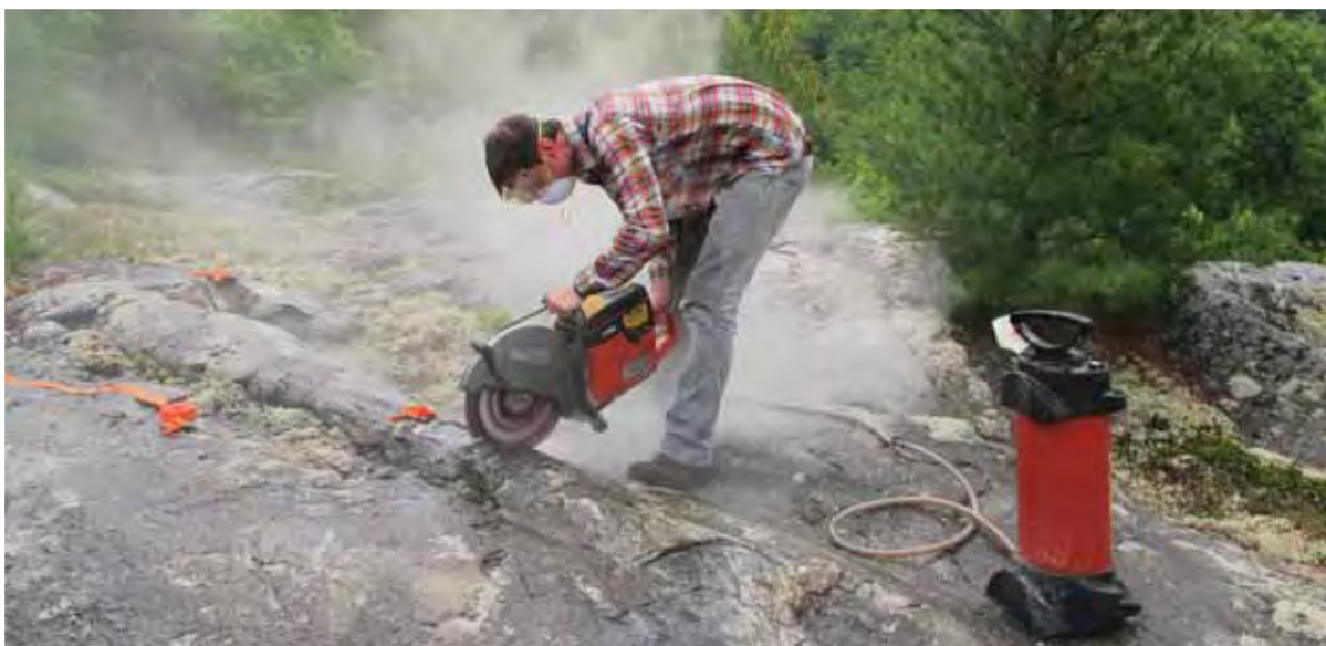
John de Bruyn (Rhodes Geology MSc student) cuts samples of partially melted mylonitised pseudotachylite from rocks cooked by one of the Earth's largest and oldest meteorite impacts, near Sudbury, Canada, using a water cooled rock saw.
