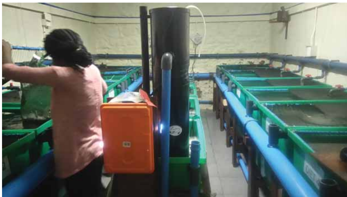
Above and left: Nyiko Mabasa's Recirculating aquaculture system, built for experiments on dusky kob nutrition.
