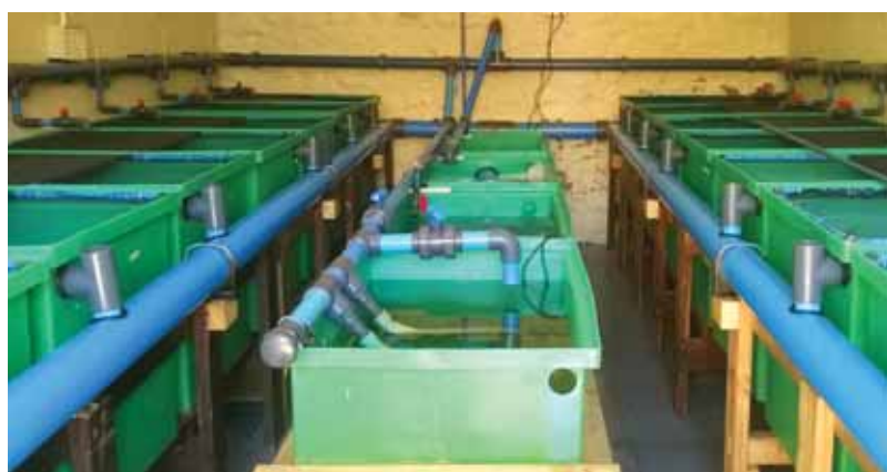
Above and left: Nyiko Mabasa's Recirculating aquaculture system, built for experiments on dusky kob nutrition.
