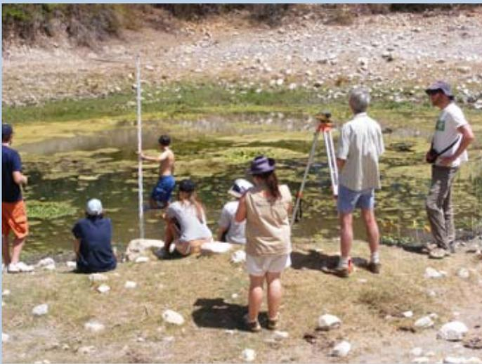
Figure 4: Students using a dumpy level and staff to measure water levels before and after pumping at the Zandvlakte well
