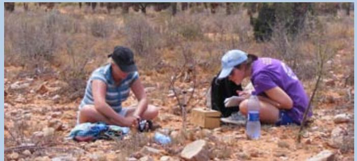
**Figure 8: Students measuring infiltration rate of water in a region of degraded thicket in the Baviaans River catchment.**
