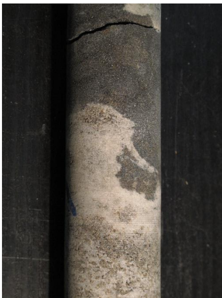
Irregular and delaminated chromitite with anorthositic footwall in core, MG-group, Eland Mine, W. Bushveld.
