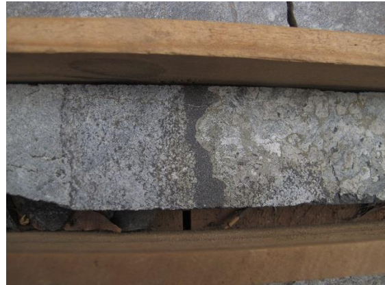
Chromitite seam with pegmatoid in pyroxenite, Uitkomst Complex, Mpumalanga.
