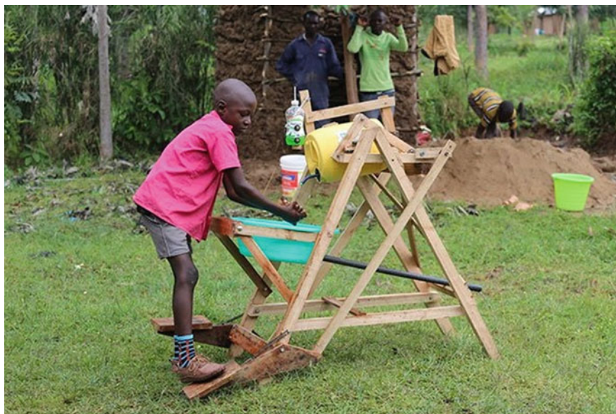
The demonstration of the no-touch hand-washing machine (Photo of Stephen Wamukota with his invention; https://str8talkmagazine.com/wp-content/uploads/2020/06/boy2-pic-data.jpg )
