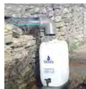
Measuring the discharge rate at the Fairview Spring
