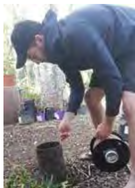
Mr Kyle Smetherham measuring the water-table in a borehole using a dip metre probe
