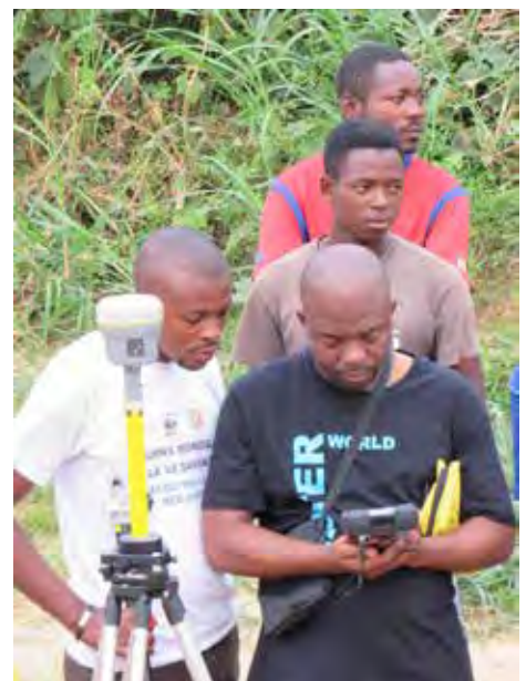
GNSS Trimble R10 measuring X, Y, Z values of the Congo River banks
