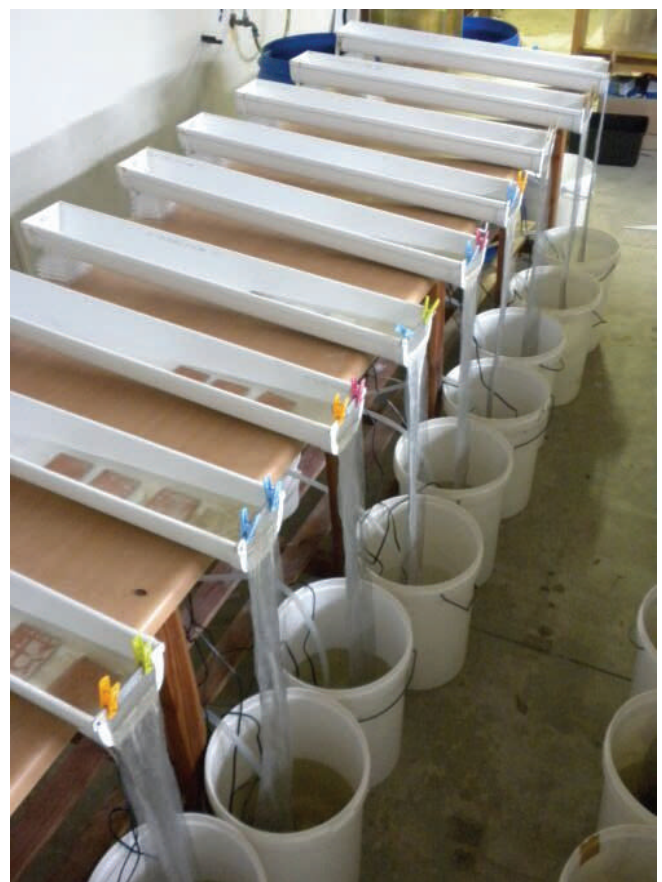
Suspended sediment exposure-response test exposing mayfly Tricorythus discolor to kaolin.
