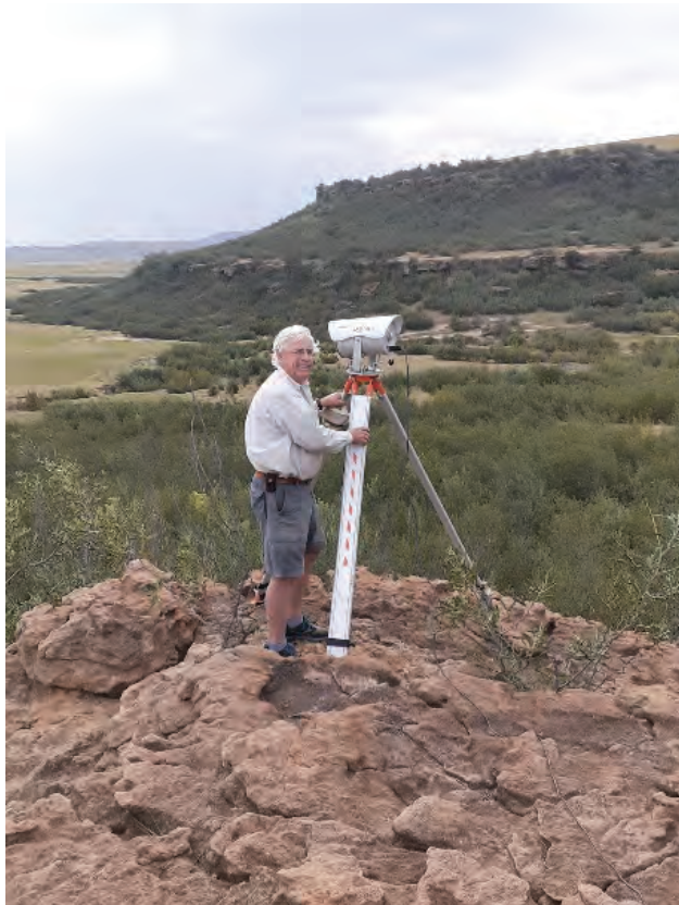
Prof. Tony Palmer installing the larger aperture scintillometer, with wattle invasions of hillslope seeps clearly visible in the background.
