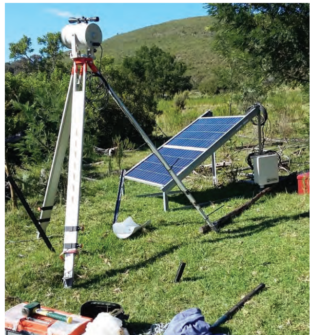
Scintillometer installed in the field by Prof Tony Palmer for measuring evapotranspiration
