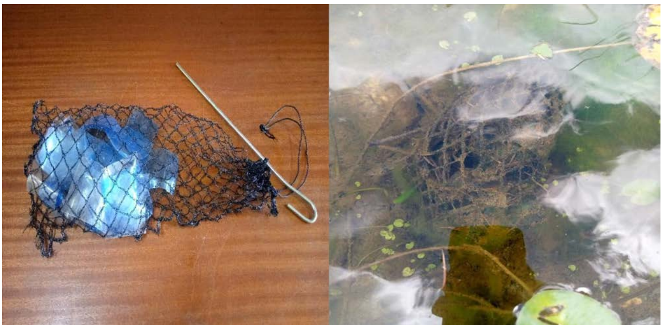
Figure 2: Macroplastic before deployment (left) and submerged (right) in the river.
