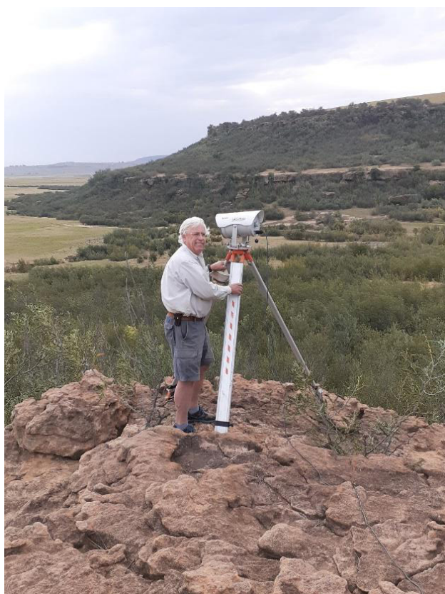
Figure 1: Prof. Tony Palmer installing the larger aperture scintillometer, with wattle invasions of hillslope seeps clearly visible in the background.
