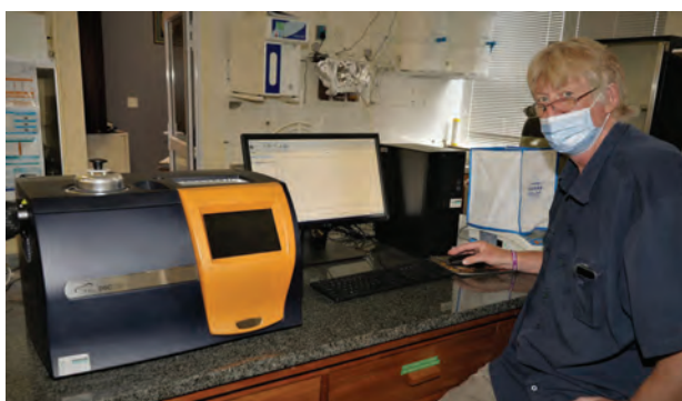
Professor Walker with the recently installed Differential Scanning Calorimeter which is used extensively by postgraduates in the Faculty of Pharmacy.
