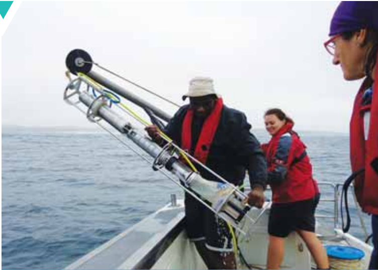
ABOVE: MSc student, Siphelele Dyantyi, and Postdoctoral Research Fellow, Dr Paula Patrick, deploy a plankton pump from the ACEP coastal research vessel, R/V uKwabelana, using a motorised winch. Principal Investigator, and NRF-SAIAB Senior Scientist, Dr Francesca Porri, looks on. Photo: Harold Marchand.
