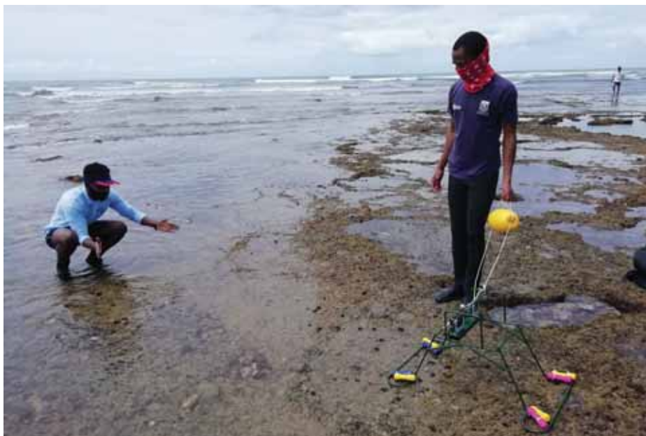
Masters students Mihle Gayiza and Them bani Mkhize setting up stereo remote underwater video systems (sRUVs) to record fishes at Flat Rocks, Gqeberha.
