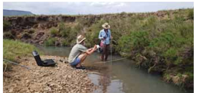
Pippa Schlegel (PhD candidate) collecting river flow data along the Minnehaha floodplain wetland, Eastern Cape.
