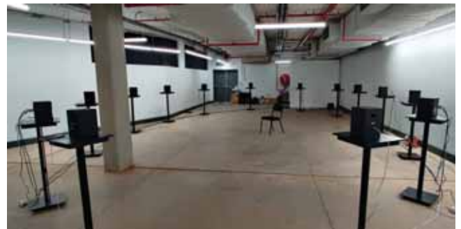
A multi-speaker configuration that was used to move wing-beat sounds of mosquitoes around a venue space. Computer programs were used to transform these sounds, arrange them into a composition, and to control their time-dependent mix levels. This was a joint project with the University of Pretoria Fine Arts and Music Departments, and was intended to promote the work of the Malaria Research Institute. Photo: Department of Computer Science
