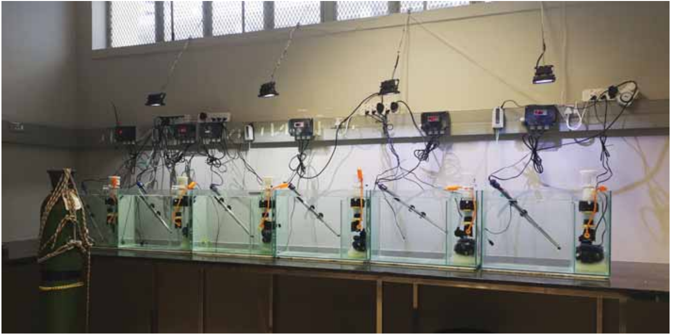
Experimental holding tanks at the NMU Ocean Science Campus, used by NRF-SAIAB researchers and students to test the impacts of ocean acidification treatment levels on larval and juvenile coastal fishes. Photo: Carla Edworthy.
