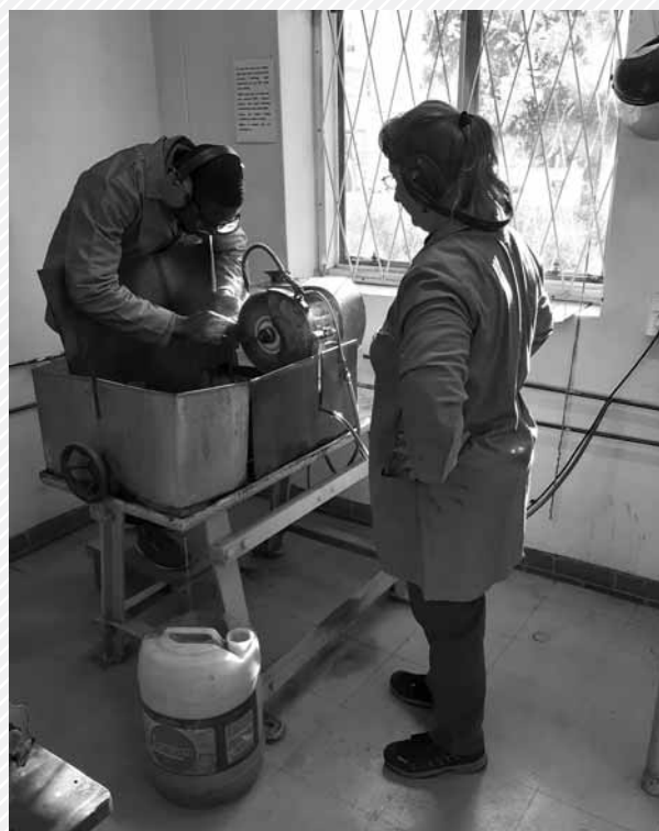
Ronald Samokomva, a first year student in Geology, being trained by Chief Technical Officer Andrea King to cut rocks using a diamond-hardened water-cooled rock saw, for research projects in the Department of Geology Credit: Steve Prevec
