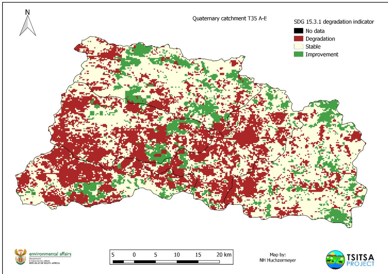
FIGURE 24: LAND AREAS IN CATCHMENT T35 A-E THAT HAVE REMAINED STABLE, ARE DEGRADED OR HAVE IMPROVED ACCORDING TO SDG INDICATOR 15.3.1.
