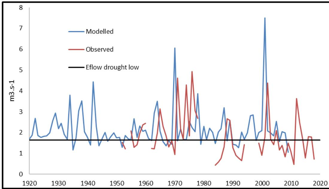
FIGURE 7: MODELLED AND OBSERVED MINIMUM ANNUAL MONTHLY FLOW DATA FOR THE TSITSA AT XONKONXA. THE EFLOW FOR DROUGHT LOW FLOWS (HIGH RISK OF FAILURE PREDICTED FOR SOCIOECOLOGICAL SYSTEM) IS INDICATED BY THE BLACK HORIZONTAL LINE
