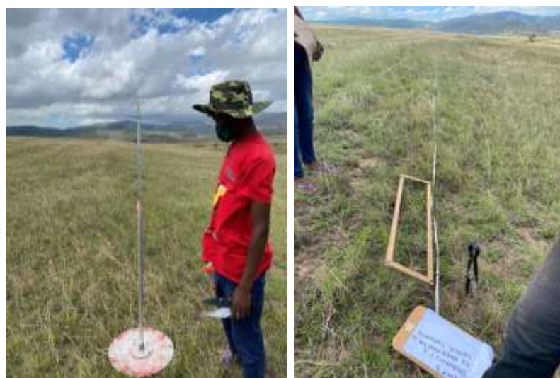
Figure 2: Left - Ecoranger assisting with estimating standing biomass using a Disk Pasture Meter; Right - A 50m transect used to estimate vegetation cover in a rested camp in Upper Sinxaku.
