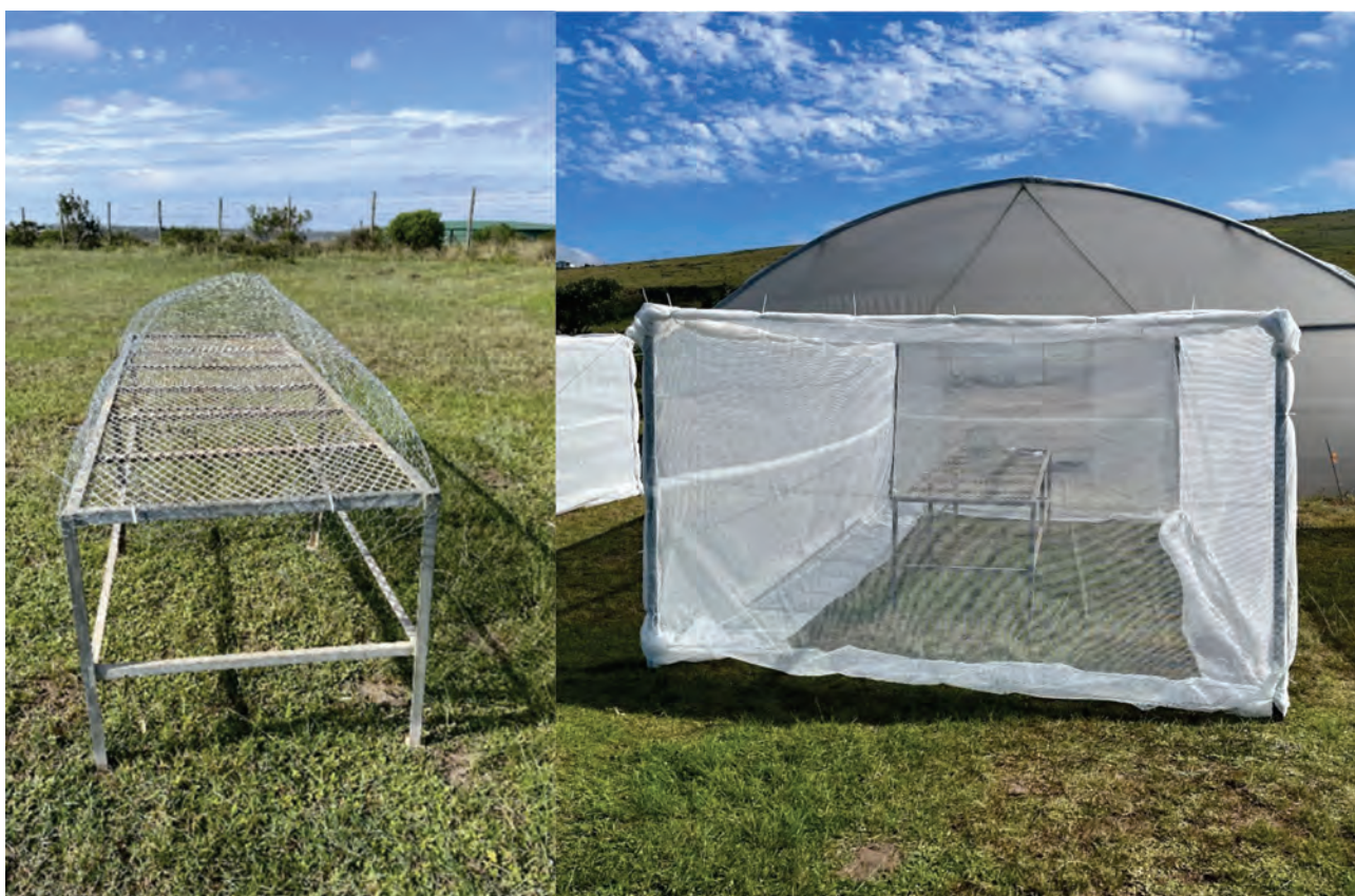
Figure 90. Netted cage and non-netted structures where the semi-field exposure of CrleGV-SA was conducted. Chicken wire was placed on top of the galvanised table to prevent birds and small mammals from interfering with the experiments. Photos: Kurhula Luphondo.
